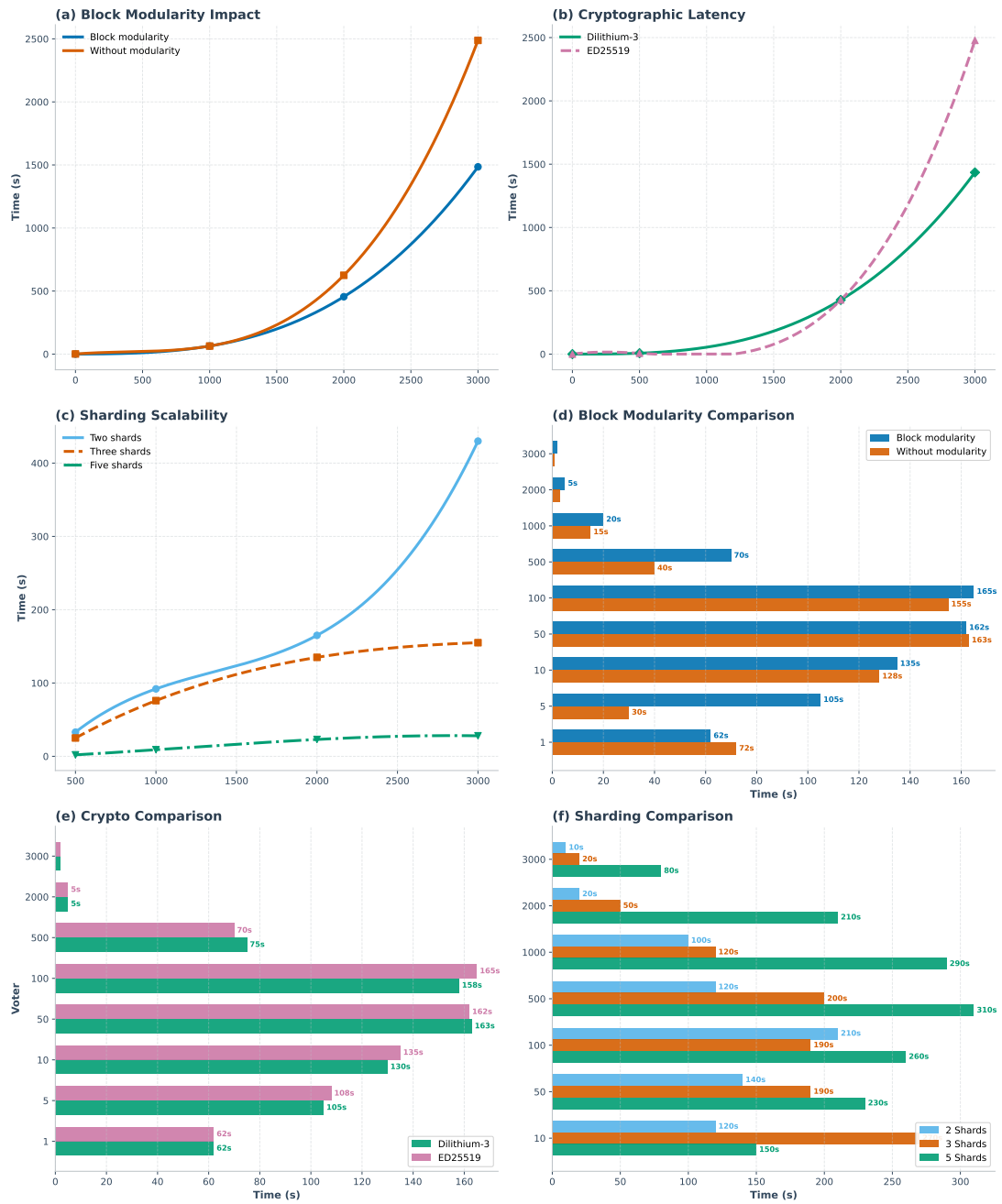
Fig. 8 The figure illustrates the visual representation of block generation time and throughput of the blockchain networks. In the representation, 'a' signifies the block generation time with and without block modularity, 'b' denotes the block generation time of Dilithium-3 and Ed25519, and 'c' represents the block generation time of sharding with two, three, and five shards. Additionally, 'd,' 'e,' and 'f' indicate the respective throughputs.
